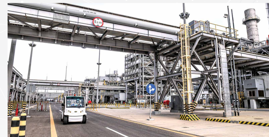
Operator Abdulmohsen O. Dawshi drives one of the Jazan Refinery Complex's electric utility vehicles inside the integrated gasification combined cycle plant's power block unit. The EVs, used by Jazan since 2019 can safely go where light vehicles are too big. The electric vehicle takes 6-8 hours to charge, and lasts about 12 hours.
